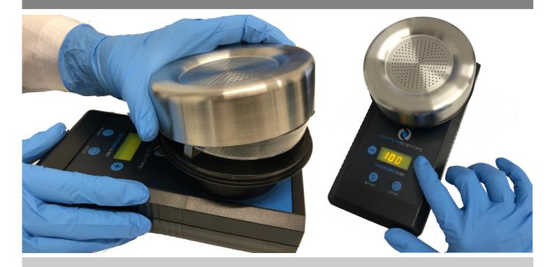
Bioaerosol samplers are vital equipment for use in bioaerosol research, clean rooms, pharmaceutical validation, food production and packaging, indoor air quality monitoring and throughout hospitals wherever air hygiene is paramount. Designed to meet the requirements of ISO14698 and ISO17141, the MicroBio MB1 Bioaerosol Sampler has a host of features making it ideal for use in such applications.
