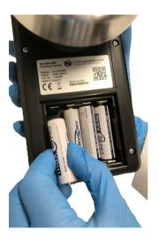
Carefully replace the lid with an upwards sliding motion ensuring the "OPEN" marking on the lid is towards the serial number label.
