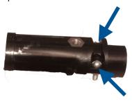
4. Solder cable onto connector pins. The connector body has pin numbers embossed onto the surface adjacent to the pins.
