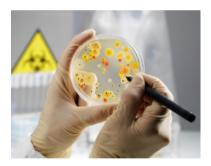
Once incubated, the colony growths are then counted, either manually or using an automatic colony counter. Due to the statistical nature of the sampling method and the chance more than one colony impinged at one point on the dish, a count correction needs to be performed.
