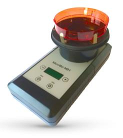
90mm petri dishes, but only the centre 55mm of the petri dish will collect samples. Using the 400 hole<sup>†</sup> sampling head will give nearly full coverage of a 90mm petri dish, improving reliability of counts.
