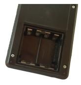
The battery is held in a small compartment at the back of the MicroBio. The unit is supplied with 4 x AA NiMH cells. The cells must be removed for re-charging in the charger supplied.
