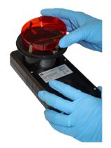
The standard MicroBio MB2 can use 220 or 400 hole sampling heads. The 220 hole sampling head can be used with both 55mm / 65mm contact plates or 90mm petri dishes, but only the centre 55mm of the petri dish will collect samples. Using the 400 x 0.7mm hole sampling head will give nearly full coverage of a 90mm petri dish, improving reliability of counts.
