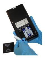
The orientation of the cells is indicated within the battery compartment.
